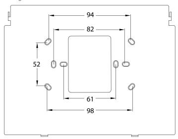
Attach the mounting plate to the wall. Hook the device to the mounting plate after all connections are done and fasten it with two screws at the bottom.
