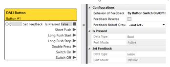
"Feedback" Portin: For all button types to give feedback based on the block's incoming "Set Feedback" port.
