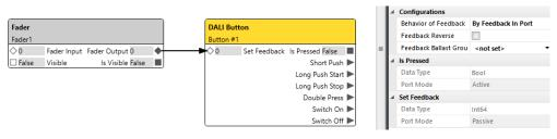
Feedback Reverse: Enable to inverse the Feedback commands: on an "activate feedback" command, the feedback is stopped ( LED off). On a "stop feedback" command, the feedback is activated (LED on).
