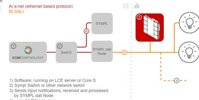
each input ("instance") informs about changes by using so called "input notifications". These event-messages can be evaluated by other controllers on the DALI line e.g. as trigger for commands sent to luminaires.
