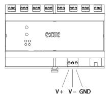
Turn the power on when all cables are connected to the SYMPL essential 2Node. The device starts operating. The device is in operation when the LED Status is flashing.
