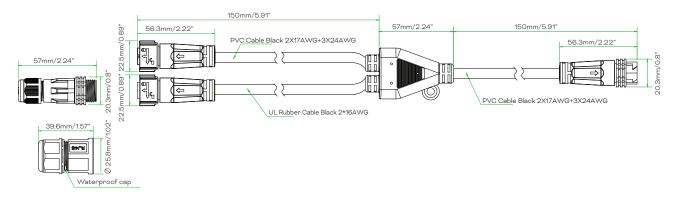
RJ45 Power Injector Cable Kit (Connector included)
