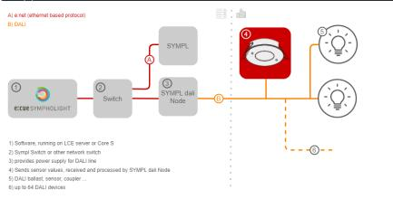
Integration in a system with DALI-2 compliant central control unit.
