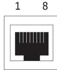
The onboard 16 VDC can be used to supply power to a DMX controller from the DMX IN RJ-45 connector. The DMX2CC has an active DMX signal repeater which eliminates the need of DMX splitter/repeaters when daisy chaining DMX2CCs.
