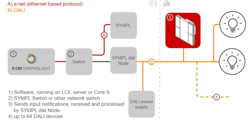
The SYMPHO DALI2 Panel 4-Key provides 4 instances (1 - 4) of type 1 (IEC62386-301, Input Devices - Push Button) which are assigned to the 4 button inputs.
