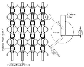
NOTE: The Mounting Bracket is designed to fit to this Ferrule dimension.
