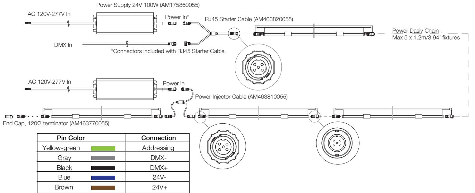
NOTE: The Address wire only needs to be connected during address configuration, it is not needed during operation. Wiring diagram shows only typical connections. Max. number of fixtures is based on minimal interconnection lengths. Actual number of fixtures is dependent on cable interconnections. Number of fixtures will reduce if longer cable lengths are used. Consult with your regional sales office to confirm maximums.
