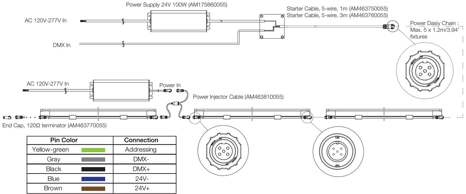
NOTE: The Address wire only needs to be connected during address configuration, it is not needed during operation. Wiring diagram shows only typical connections. Max. number of fixtures is based on minimal interconnection lengths. Actual number of fixtures is dependent on cable interconnections. Number of fixtures will reduce if longer cable lengths are used. Consult with your regional sales office to confirm maximums.
