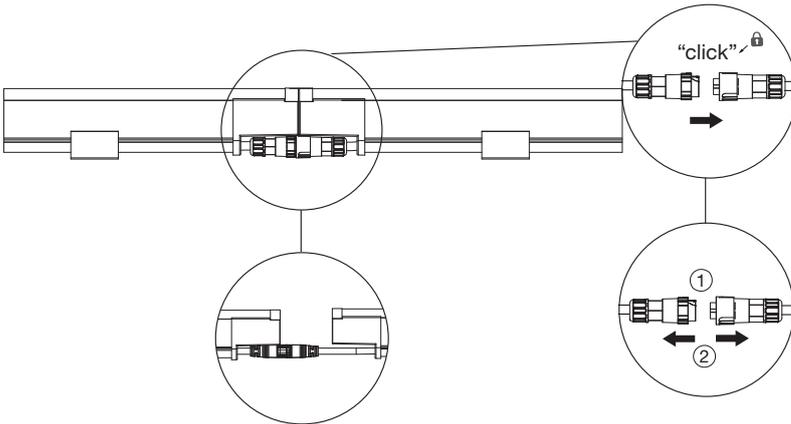
If you do not hear "click", rotate the spring loaded connector manually to ensure that the connectors are properly mated.
